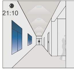
21:10 The light dims to stand-by level after the hold-time.
