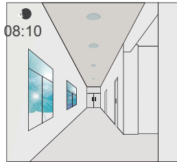
08:10 When the natural light level exceeds setpoint off to light, the light will turn off even if when the space is occupied.
